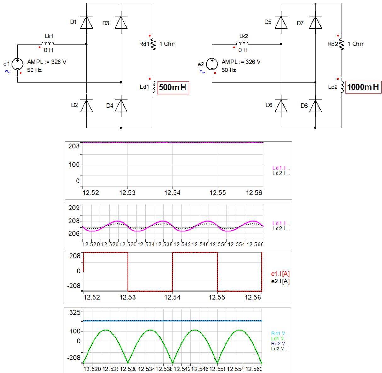
Load inductance does not affect the average load current, but only its ripple.
