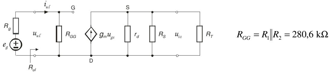
$$R_{ul} = \frac{\dot{U}_{ul}}{\dot{I}_{ul}} = R_{GG} = 280,6 \text{ k}\Omega$$
